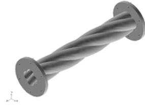
Fig. 2 Optimized swirl pipe geometry
